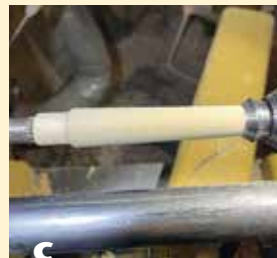
(b) Outboard side: Locking pliers grip the lamp rod next to the wood centering plug, preventing the rod from rotating with the spindle. (c, d) Turn a wood Morse taper to fit your lathe. Drill all the way through the wood MT.
