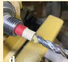
(b) Outboard side: Locking pliers grip the lamp rod next to the wood centering plug, preventing the rod from rotating with the spindle. (c, d) Turn a wood Morse taper to fit your lathe. Drill all the way through the wood MT.
