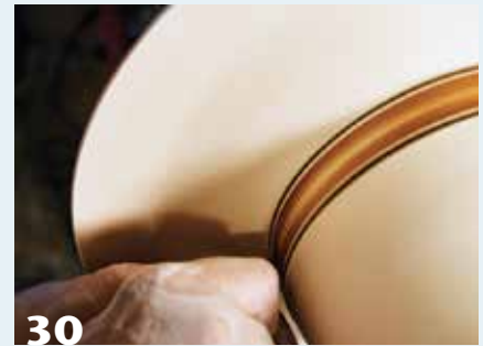
A strip of exotic hardwood is pressed on the spinning hatband, burnishing the wood and mimicking an applied band.
