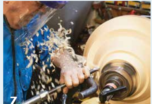
(6) With the blank mounted on a screw chuck, form a tenon at the top of the crown, then mount a chuck on the tenon and ensure it runs true. This ensures centeredness when the hat is reverse-mounted later.
