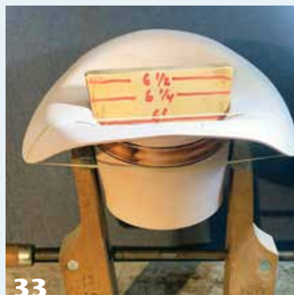
With the hat in a screw clamp, a stop block defines the final interior width, and heat from a lamp "bakes" it dry in this position.
