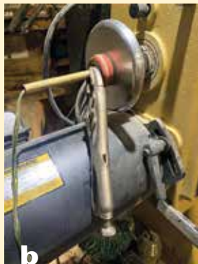
(b) Outboard side: Locking pliers grip the lamp rod next to the wood centering plug, preventing the rod from rotating with the spindle. (c, d) Turn a wood Morse taper to fit your lathe. Drill all the way through the wood MT.
