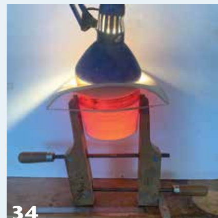
With the hat in a screw clamp, a stop block defines the final interior width, and heat from a lamp "bakes" it dry in this position.
