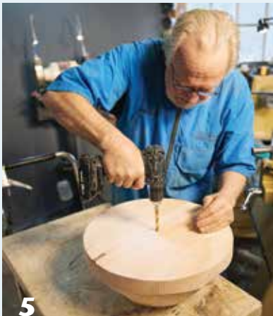
Pre-drill the bottom side for mounting on a screw center. Note the extra band of material at the widest part, which allows you to adjust the position of the hat in the block if needed.
