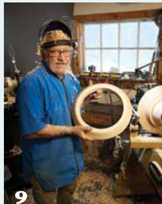
The author opts to part a ring of wood, rather than waste it. The rings make great mirror frames.
