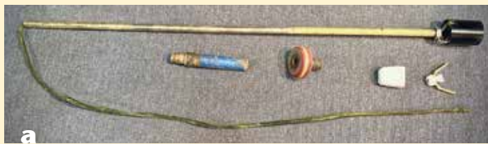
(a) Light rod components, all purchased, except for the wood Morse taper and outboard centering plug.
