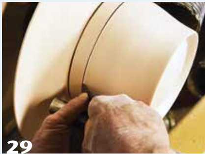
A strip of exotic hardwood is pressed on the spinning hatband, burnishing the wood and mimicking an applied band.
