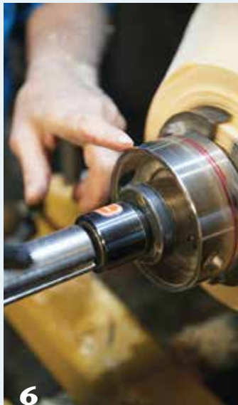
(6) With the blank mounted on a screw chuck, form a tenon at the top of the crown, then mount a chuck on the tenon and ensure it runs true. This ensures centeredness when the hat is reverse-mounted later.
