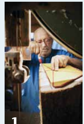
1 Mark the block's endgrain using a sizing/positioning template.
