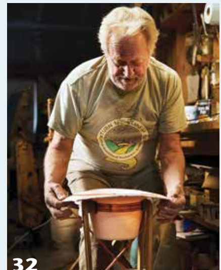
The hat is set in a bending jig, whose curved jaws squeeze the band into an oval shape. Rubber bands pull the brim into the desired curve.
