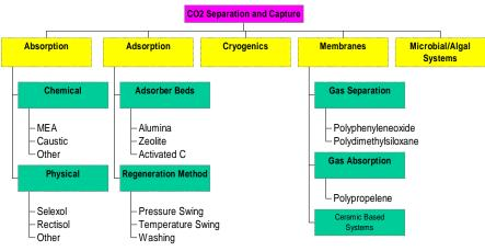
Figure 1. Technology Options for CO<sub>2</sub> Separation and Capture
