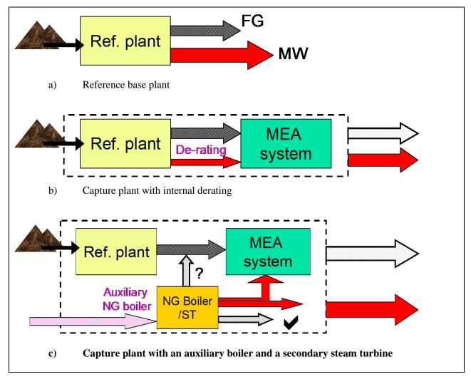
In terms of the configuration of the  $CO_2$  capture system shown in Figure 3, the user can make the following choices as well
