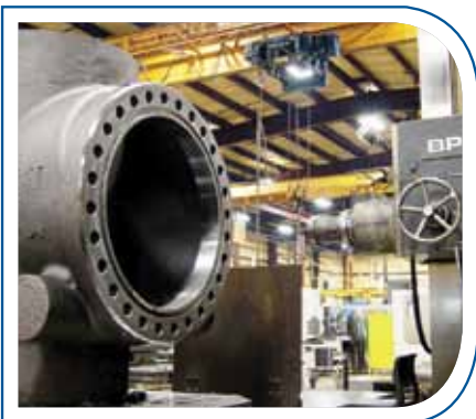
Oil Field pipeline valve: Cast by Bradken and finish machined by Bradken
