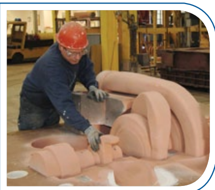
Molding/core making (complex pump housing)
