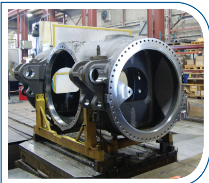
Large, machined steel differential for mining truck
