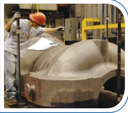
Large steel turbine housing
