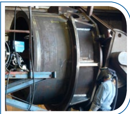
Heavy fabrications using weld positioners
