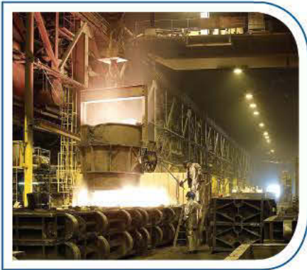
Large steel castings to 55,000 lbs. AOD capable
