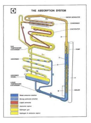
hydrogen free to rise through the absorber coil and to return to the evaporator. The hydrogen thus circulates continuously between the absorber and the evaporator.
