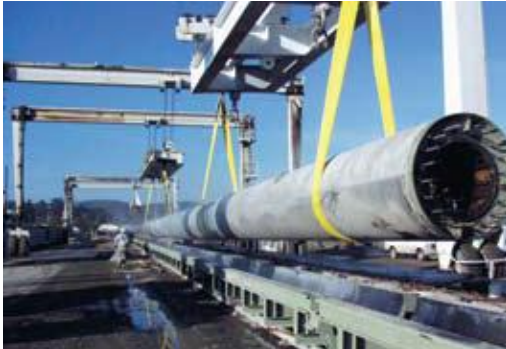
4500 precast concrete piles were driven into difficult soil conditions to create the foundation for the 1.7 million square-ft Boston Convention & Exhibition Center in South Boston, Mass. Architect: HNTB and Rafael Vinoly Architects (a joint venture).
