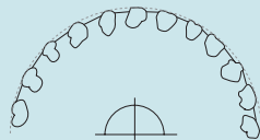
AFTER DRESSING THE WHEEL FACE IS OPEN WITH THE GRITS EXPOSED, READY FOR EFFICIENT GRINDING ACTION
