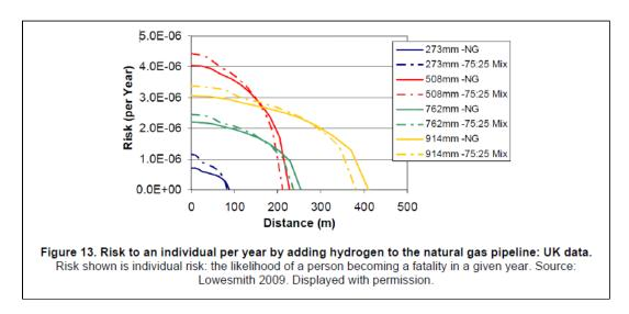
Figure 28. Risk to an individual per year by adding hydrogen to the natural gas pipeline: UK data.
