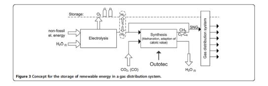
Figure 30. Methanation Concept for producing renewable methane from electrolytic hydrogen and CO<sub>2</sub> <sup>91</sup>.
