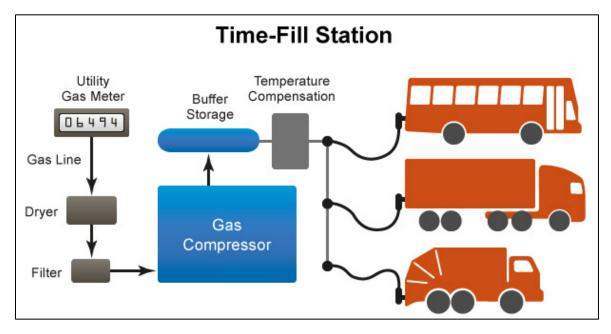
Figure 9. CNG Time fill station configuration
