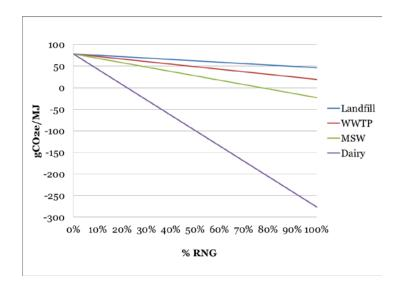
Figure 23. Change in CI values of fossil CNG when increasing the percentage of renewable CNG in the blend.
