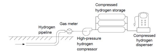
Figure 16e. Hydrogen station with hydrogen pipeline delivery.
