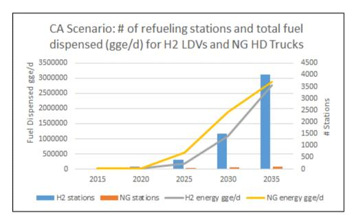
Figure 31. Number of station and fuel use in long-haul NG truck and H2 FCV scenarios.
