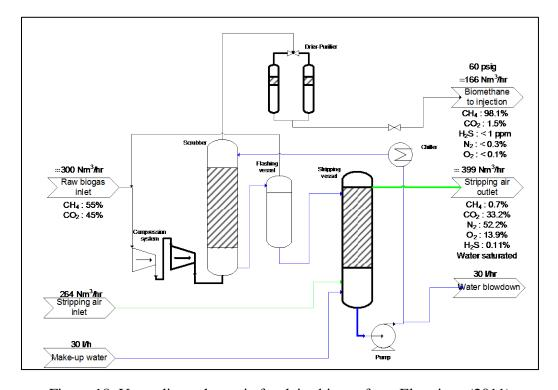
Figure 18. Upgrading schematic for dairy biogas from Electrigaz (2011)
