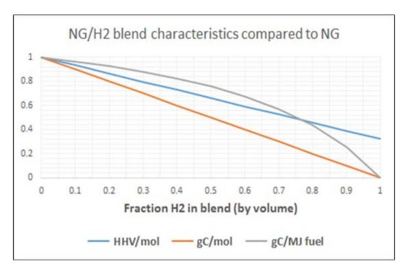
Figure 29. Effect of blending green hydrogen with natural gas on fuel gas energy and carbon content. The y-axis shows the fraction compared to pure natural gas.
