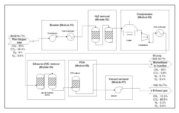
Figure 19. Upgrading schematic from LFG from Electricgaz (2011).
