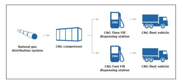
Figure 8. CNG supply pathway
