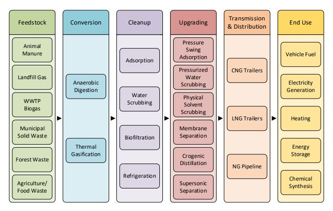
Figure 16: Schematic of RNG production from feedstock through to end use.
