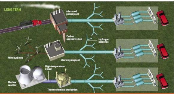
Figure 14. Near Term and Long Term Pathways for Hydrogen Production and Delivery to Vehicles. (It is also possible to deliver hydrogen via compressed gas truck.)
