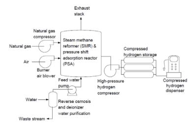
Figure 15a. Hydrogen refueling station with onsite steam methane reforming.
