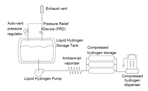
Figure 16d. Hydrogen station with liquid hydrogen delivery.
