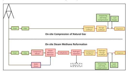
Figure 25. Onsite H2 Production Pathway Comparison to a Conventional CNG Station
