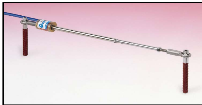
Figure 5.6 - Geokon Model 4420 Displacement Gage
