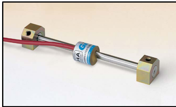
Figure 5.4 - Geokon Model 4000 Strain Gage
