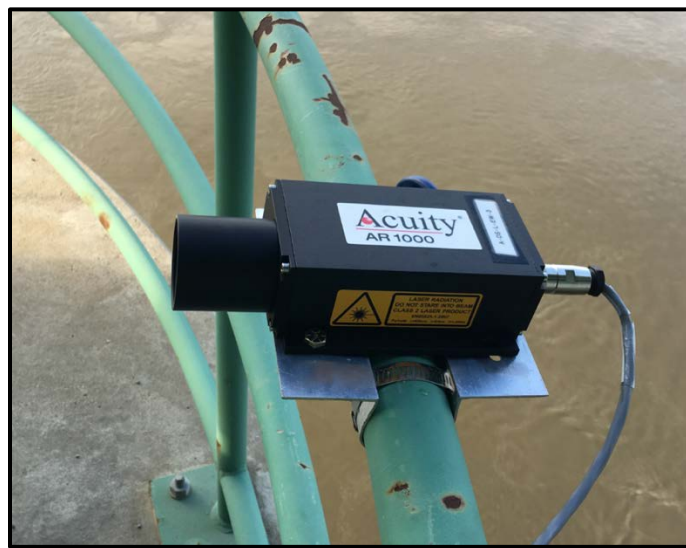
Figure 6.9 - Acuity AR1000 Laser and Attachment
