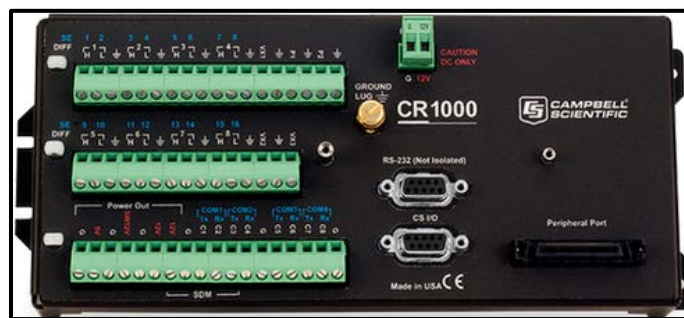
Figure 5.7 - Campbell Scientific CR1000 Datalogger
