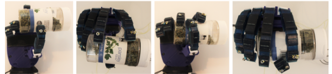
Fig. 8. A switch from pinch to power grasp. The first two images depict the pinch grasp and the last two images the power grasp. The execution of this task is facilitated by the finger interdigitation.
