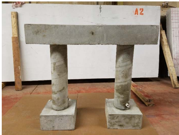
(f) Grouted bent and concrete filled cap beam
