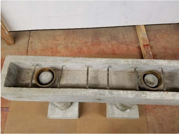
(c) Assembled precast pier
