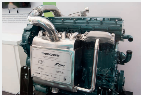
Dolphin N2 recuperated split cycle engine demonstrator
