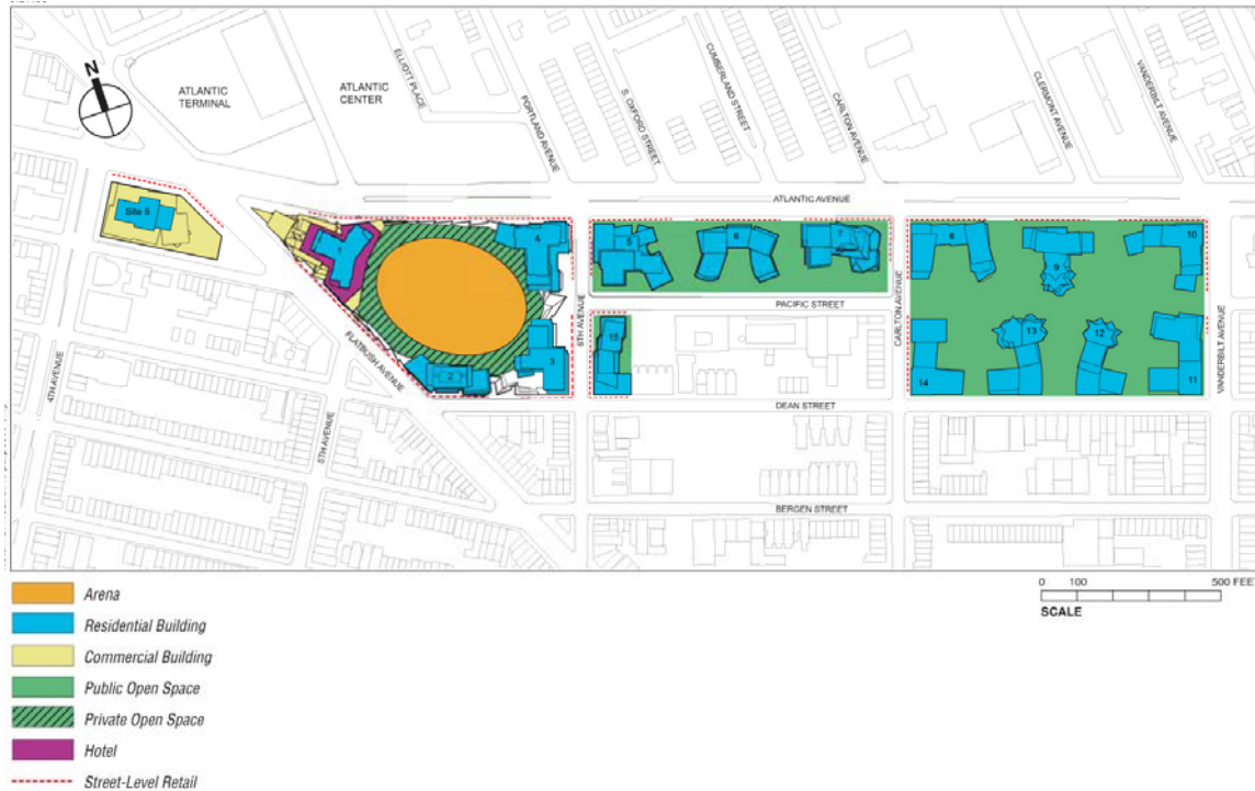
FIGURE 37. Site plan showing arena, open space, configuration of buildings, and organization of superblocks at the proposed Brooklyn Atlantic Yards project, 2006.
