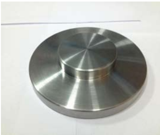
Figure 10 Example of pre-machined blank of a flatness-of-surface test piece.
