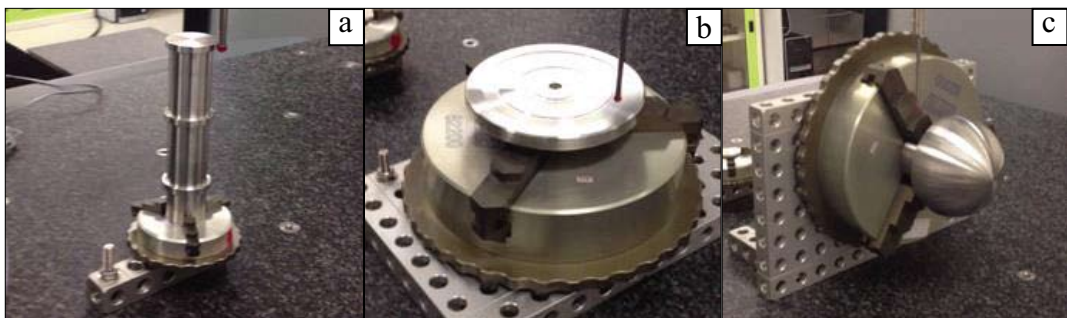
Figure 11 Measurement of test pieces using the coordinate measuring machine: (a) Cylindrical test piece; (b) Flatness-of-surface test piece; (c) Circular test piece.
