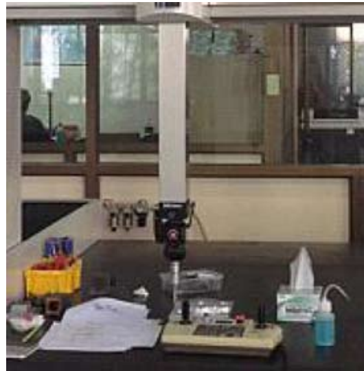
Figure 9 Measurement of the case study using the coordinate measuring machine.
