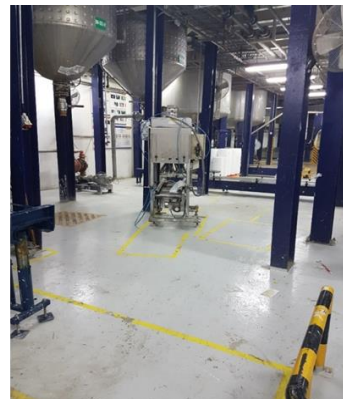
Fig. 7. Floor marked as per the filling size packing.
