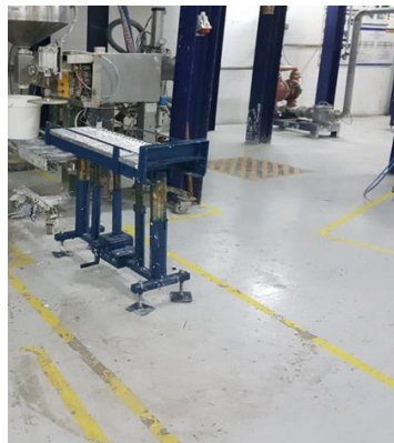
Fig. 7. Floor marked as per the filling size packing.
