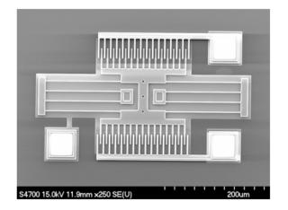
Figure 17: MEMS Strain Gauge
