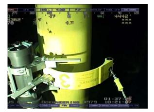
Figure 15: Deep water Pipe Pressure Sensor<sup>50</sup>
