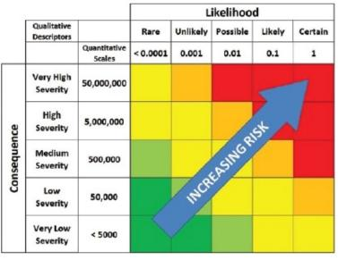
Figure 4: Example of a 5x5 risk matrix using log-log quantitative scales.
