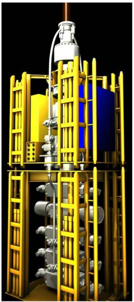
Figure 9: BOP Stack<sup>43</sup>
