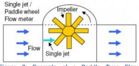
Paddle Figure 7: Example of а Type Flow Measurement Device<sup>38</sup>
