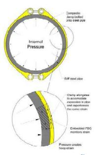
Figure 14: FBG for Pressure Sensing<sup>50</sup>
