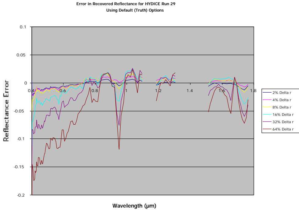
Figure 4.1-2. Plot of reflectance error for the inversion to reflectance using the truth (default) data from the time of acquisition .
