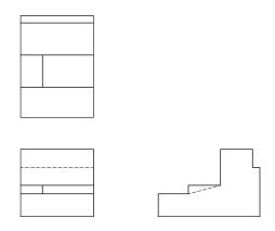
Figure 2. An example of a formal multiview drawing. Note that in multiview engineering drawings the views are not labeled; the placement and alignment communicates the relative viewpoints.
