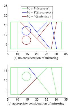
Figure 6. (a) Even if we align the two views in terms of scale and translation, it is not easy to compare them at a glance; here half the elements still appear to be slightly off. (b) In fact, most elements match perfectly if the correct affine transformation is applied. The real problem is mirroring and two lines that only partially differ.
