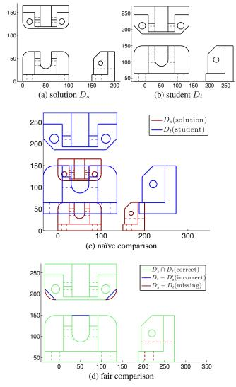
Figure 8. Comparing the solution to a student's drawing. To be compared to  $D_t$ , all views in  $D_s$  are scaled 1.7 times larger. The top, front, and right views are translated (-33.8, +186.2), (-33.8, +39), and (+187.7, +39), respectively. All views have zero rotation and skew. By aligning them, the algorithm finds incorrect and missing lines, which are represented in blue and dark red.
