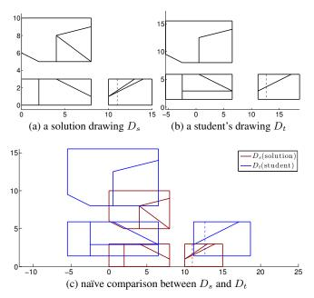
Figure 4. An example of (a) a solution drawing and (b) a student's drawings and (c) their naïve comparison. Because they have different scales, translations, and offsets, a naïve comparison does not work.
