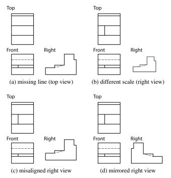
Figure 3. Four typical cases of mistakes. Note that the labels on the views are not present in the actual multiview drawing.
