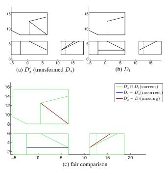
Figure 7. We estimate the transformation for each view individually using RANSAC. By applying the transformations to the views in  $D_s$ , we get the transformed version  $D'_s$ . Then the elements of  $D'_s$  and  $D_t$  can be compared one by one.
