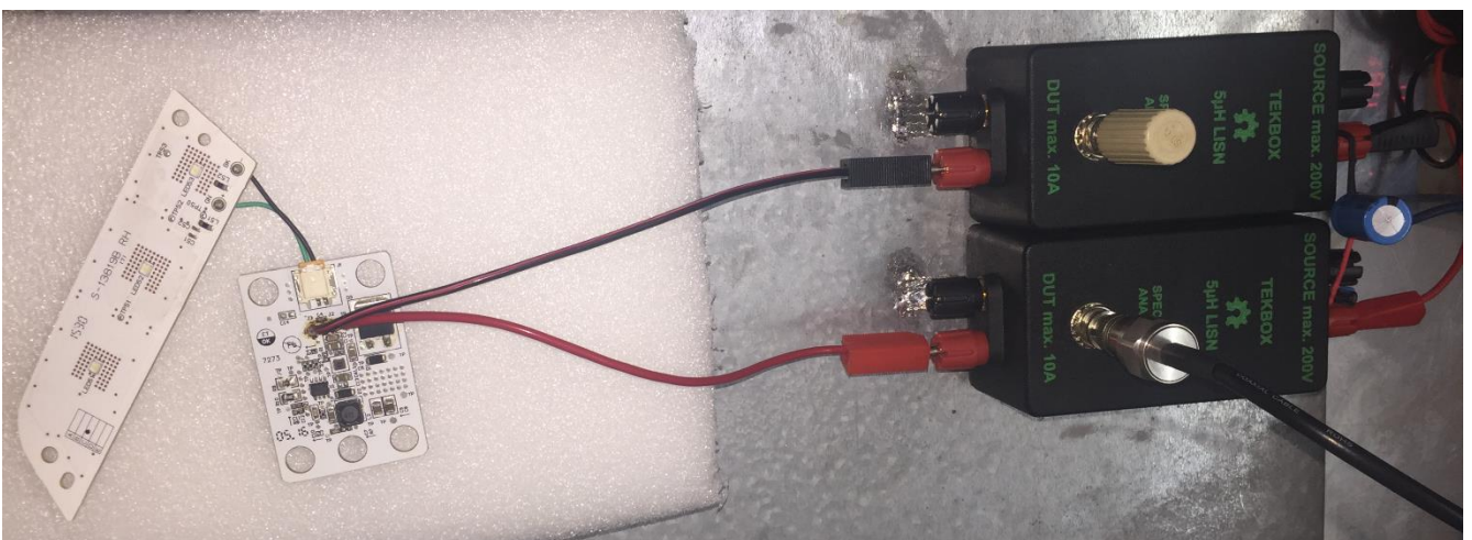
Picture 1: simple pre-compliance conducted emission measurement set up, voltage method
