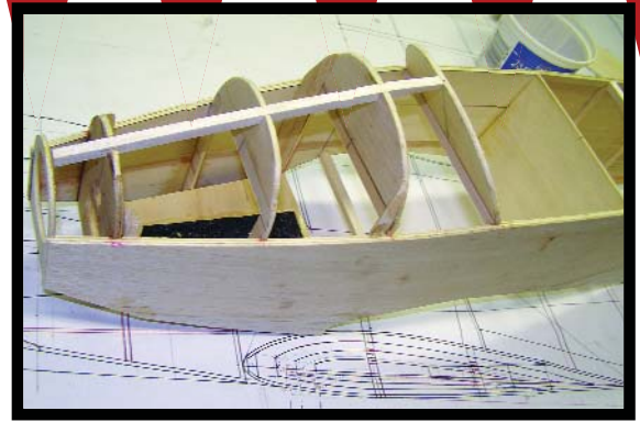
Above: The fuselage is built upside-down and then top formers are glued on. Some formers are in two sections.
