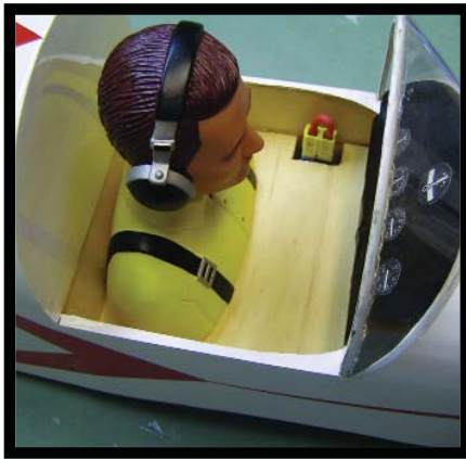
A 1/4-scale pilot can be trimmed to suit the open cockpit. A full canopy is another option. The open version hides a motor arming plug.
