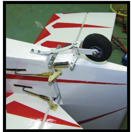
The author constructed a homemade tail wheel assembly to replicate the full-scale aircraft's. Conventional pushrods make radio setup easy.
