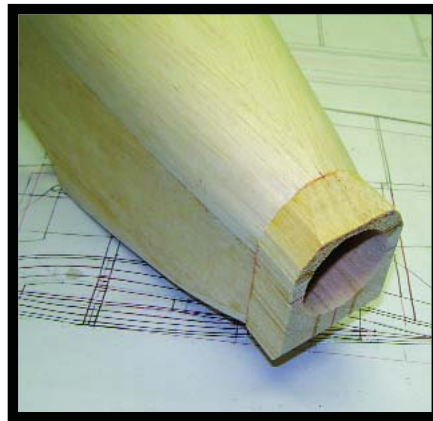
Notice the large opening in front for the motor to go through. Consult the plans for the correct contour shape of the nose block.
