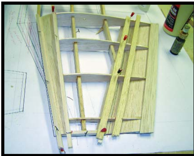
Bottom aileron sheeting is glued to the ribs and the spar. The wingtip's top LE is adhered to the ribs and to the LE.
