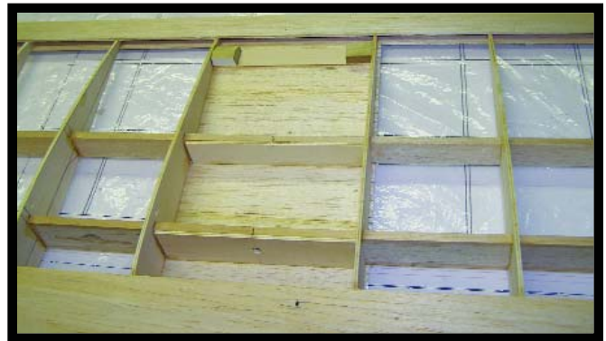
Above: The top TE is glued to the ribs. The hardwood landing gear block is glued to the ribs. Predrill the block for the \frac{5}{32} -inch-diameter piano wire.
