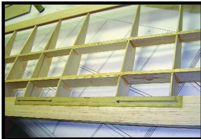
Bottom aileron sheeting is glued to the ribs and the spar. The wingtip's top LE is adhered to the ribs and to the LE.
