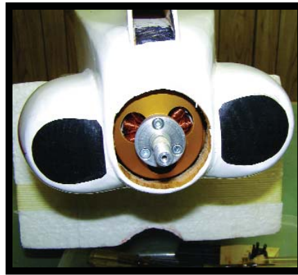
An AXI 4120/18 outrunner motor running on a 6S pack is equivalent to a .46-size two-stroke engine. An approximately 12 x 8 propeller works for this setup.
