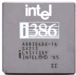
Intel 80386 DX rated at 16 MHz
