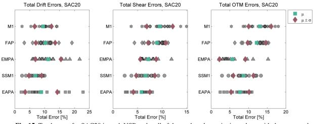
**Fig. 15.** Total errors for SAC20 in each NSP under all of the earthquake excitations along with the mean and mean +/- one standard deviation of them
