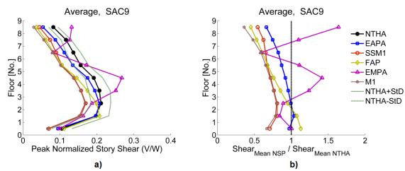
Fig. 9. a) The mean peak normalized story shear profiles and b) the peak story shear error profiles for SAC9
