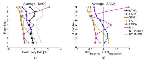
Fig. 8. a) The mean peak story drift profiles and b) the mean peak story drift error profiles for SAC9
