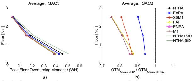
Fig. 6. a) The mean peak normalized floor overturning moment profiles and b) the mean peak floor overturning moment error profiles for SAC3
