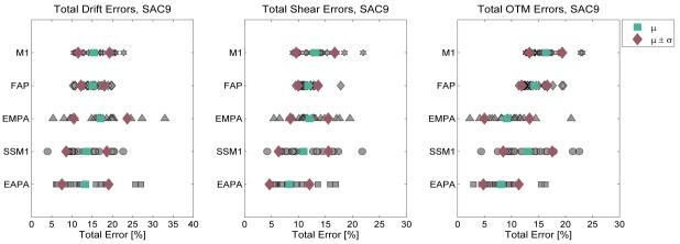
**Fig. 11.** Total errors for SAC9 in each NSP under all of the earthquake excitations along with the mean and mean +/- one standard deviation of them
