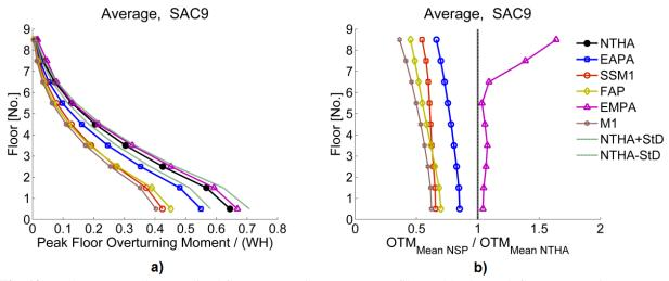
Fig. 10. a) The mean peak normalized floor overturning moment profiles and b) the peak floor overturning moment error profiles for SAC9
