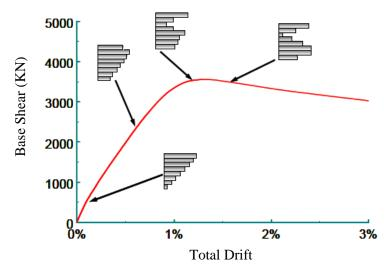
Fig. 1. The capacity curve obtained from an adaptive pushover analysis along with the applied load vectors that are updated during the analysis (Elnashai and Di Sarno, 2008)
