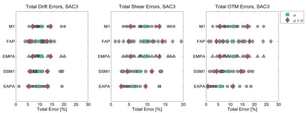
Fig. 7. Total errors for SAC3 in each NSP under all of the earthquake excitations along with the mean and mean +/- one standard deviation of them
