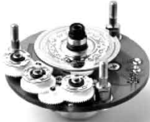
Figure 3-21 Internal construction of a multi-turn absolute encoder, photo view
