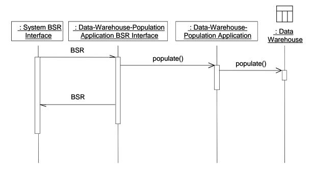
Figure 25. Push Option for Data-Warehouse Population Using BSRs
