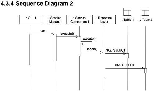
Figure 17. Sequence Diagram for a Report Executed from a Service Component
