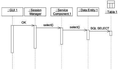
Figure 14. Sequence Diagram for Access Involving One Business Object
