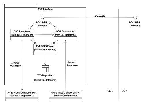
Figure 11. Elements of a BSR Interface Package
