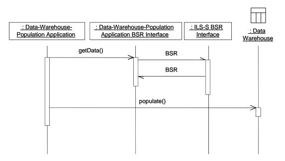
Figure 23. Pull Option for Data-Warehouse Population Using BSRs
