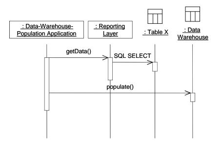
Figure 24. Pull Option for Data-Warehouse Population Using the Reporting Layer
