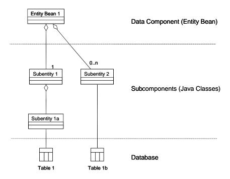
Figure 9. Data Component Internals – Aggregate Entity Pattern
