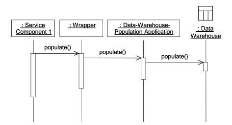
Figure 26. Push Option for Data-Warehouse Population Using a Wrapper Component
