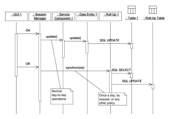
Figure 20. Sequence Diagram for a Batch Roll Up
