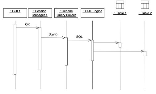
Figure 18. Sequence Diagram for an Ad Hoc Query
