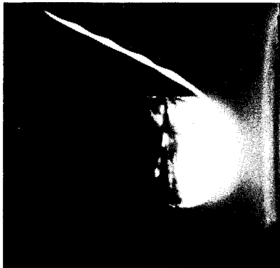
(a) Hemispherical-nose model. P_s = 2.40 \text{ atm}; K_o = 0.23 . \dot{q}_s = 700 \text{ Btu/ft}^2\text{-sec} (7.95 MW/m 2 ); H_s = 2340 \text{ Btu/lbm} (5.43 MJ/kg).
