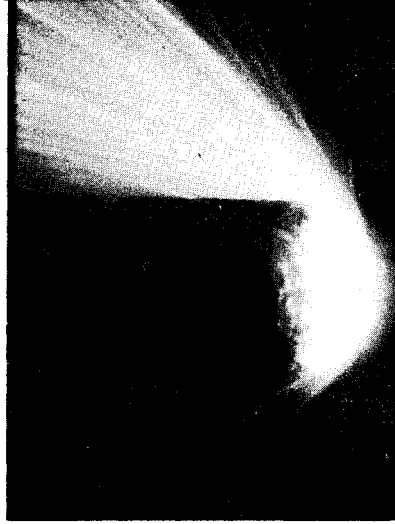
L-70-4708 (c) Hemispherical-nose model. P_s = 11.26 \text{ atm}; K_o = 0.09 ; \dot{q}_s = 620 \text{ Btu/ft}^2\text{-sec} (7.04 MW/m 2 ); H_s = 1100 \text{ Btu/lbm} (2.55 MJ/kg).
