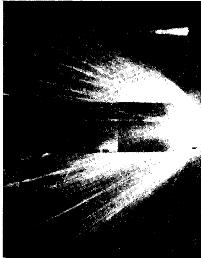
(b) Blunt-nose model. P_s = 10.41 \text{ atm}; K_o = 0.13 ; \dot{q}_s = 400 \text{ Btu/ft}^2\text{-sec} (4.54 MW/m 2 ); H_s = 1100 \text{ Btu/lbm} (2.55 MJ/kg).
