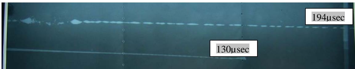
Fig2(a): Flash X-ray records of jets in air at 130 \mu sec and 194 \mu sec as produced from shaped charge of Fig.1.
