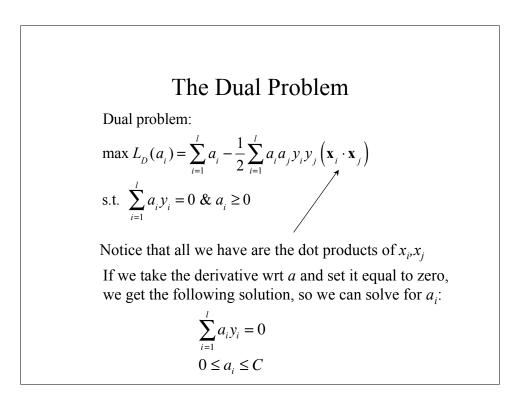
Now knowing the  $a_i$  we can find the weights **w** for the maximal margin separating hyperplane:
