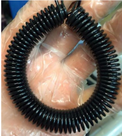
Figure 10: When a piece of copper is completely black it has anywhere between 30,000 and 40,000 layers of Nano particles.
