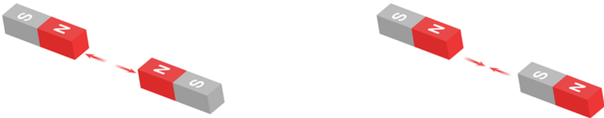
Figure 3: The image on the left shows how two magnets of the same polarity will repel from one another where the right side shows opposite polarities attracting and creating a balance.
