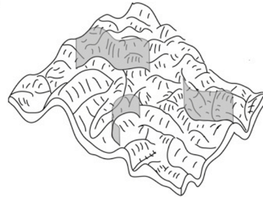
d) The relation between salt flow into a salt dome, and the formation of constriction folds and boudins.
