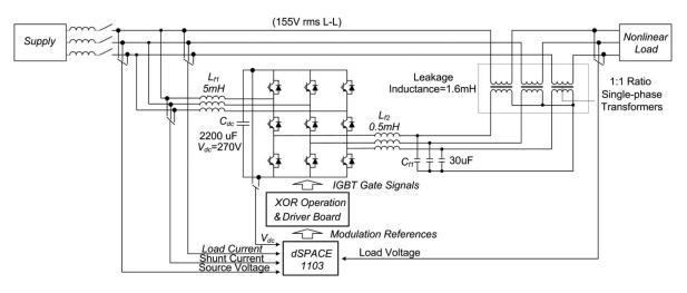
Fig. 8. Experimental setup and parameters used for testing.
