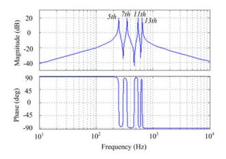
Fig. 6. Bode representation of the selective harmonic regulators found in the series control scheme.
