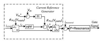
Fig. 7. Shunt control block representation.
