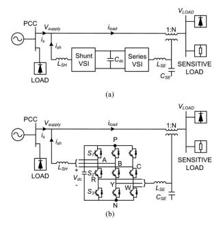
Fig. 1. Representations of (a) back-to-back and (b) nine-switch power conditioners.
