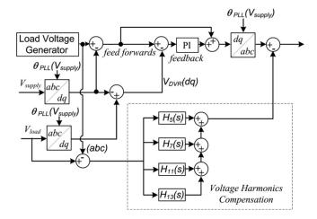
Fig. 5. Series control block representation.
