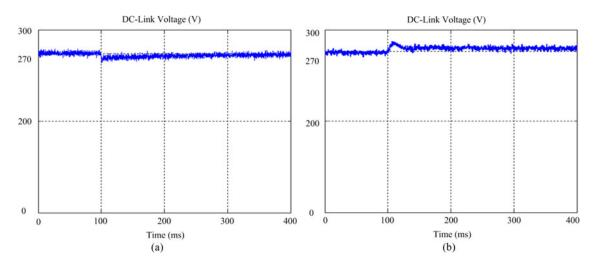
Fig. 13. Experimental dc-link voltage during (a) normal-to-sag and (b) sag-to-normal transitions.
