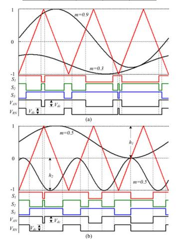
Fig. 2. Arrangements of references having (a) the same frequency but different amplitudes, and (b) different frequencies but the same amplitude.
