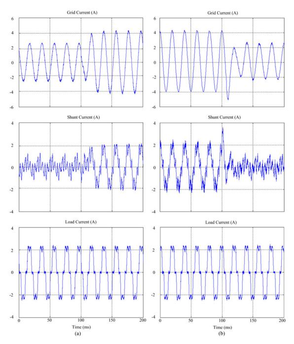
Fig. 12. Experimental grid, shunt injection, and load currents during (a) normal-to-sag and (b) sag-to-normal transitions.
