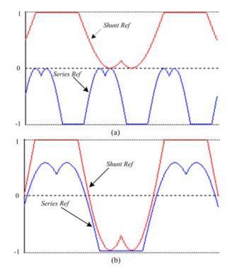
Fig. 4. 120°-discontinuous references with (a)  $M_{SH} = M_{SE} = 0.5$ ,  $\omega_{SH} \neq \omega_{SE}$ , and (b)  $M_{SH} = 1 \times 1.15$ ,  $M_{SE} = 0.8 \times 1.15$ ,  $\omega_{SH} = \omega_{SE}$ .
