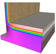
B) THERMAL IMAGE CONTOURS OF WALL SYSTEM WITH A THERMAL BREAK
