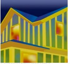
A) IMAGE SHOWING THERMAL BRIDGE DUE TO NO THERMAL BREAK AND WALL STUDS
