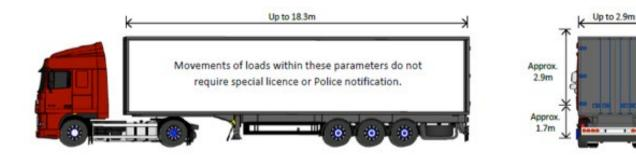
FIGURE 13 THE ROAD VEHICLES (CONSTRUCTION AND USE) REGULATIONS 1986
