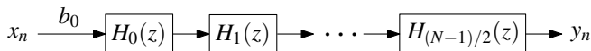
Figure 9.10. Cascade realization of a transfer function composed of an odd number of factors.
