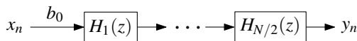
Figure 9.9. Cascade realization of a transfer function composed of an even number of factors.
