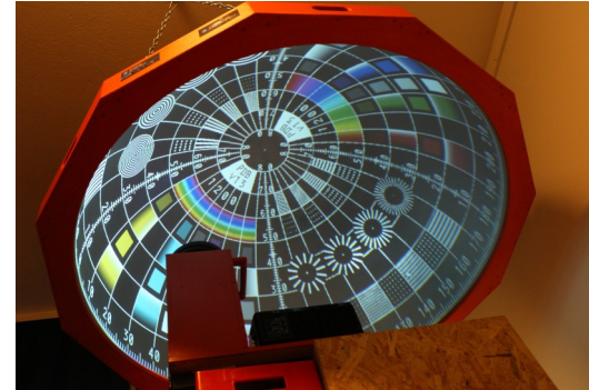
Here the projection lens is at the OFF_OUT_Y=0.5 position. It's clearly visible that the image gets brighter at the left side and darker at the right side.
