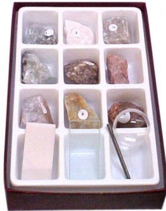
Standard Mohs testing kit, containing materials of different Mohs 1-9 in a box. Each material is clearly labelled 1-9. The kit may contain other common materials, such as glass, a penny and a nail.
