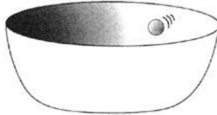
Figure 7.2 Bowl and ball bearing: a system with a stable energy state.
