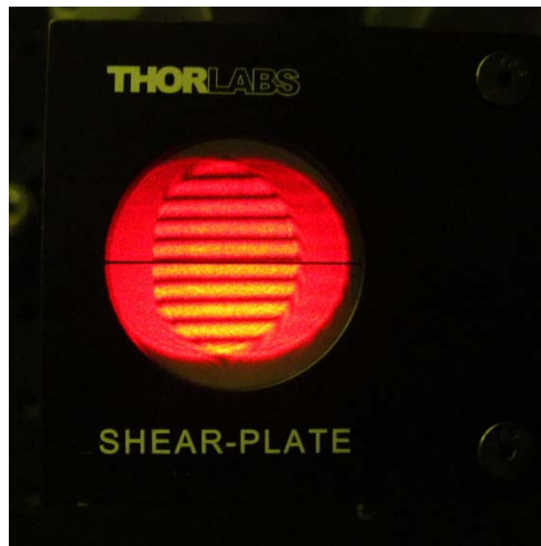
Figure 3: Shear plate interferogram for a collimated beam
