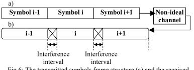
Fig.6: The transmitted symbols frame structure (a) and the received symbols are overlapping during the "interference interval"(b)
