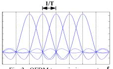
Fig. 3: OFDM transmission spectrum
