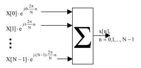
really important, the complex exponential carriers are orthogonal to each other, as we know from the Fourier decomposition. These carriers are frequency spaced with  $\Delta\Omega = 2\pi/N$ . If we consider that the N data symbols X[k] come from sampling an analog information with a frequency of f<sub>s</sub>, an easy to make discrete to analog frequency conversion indicates a  $\Delta f = 1/T$  spacing between the subcarriers of the transmitted signal. The
