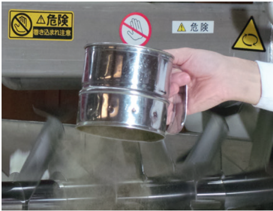
Spreading the mould spores.
