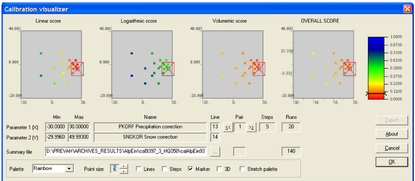
Fig. 8. VIEWOPTIM graphical user interface for visualising and verifying PREVAH calibration runs. For this, parameters are assessed pair-wise concerning their modelling efficiency.
