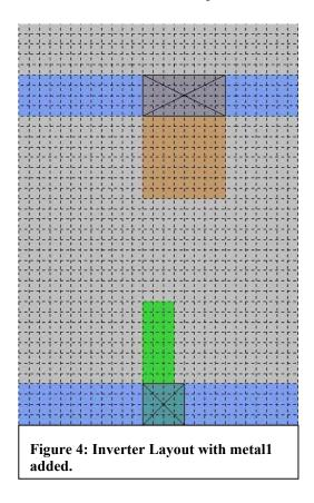
The next step is to paint the n-well area where the PMOS fet is located. Similarly for NMOS devices a p-well area should be added, although this step is not 100% necessary since MAGIC knows already that a p-well area is needed (assuming the technology process is n-well based)<sup>3</sup>. Nevertheless, it remains good practice to place the p-well layer by hand.
