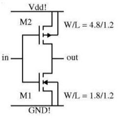
Figure 2: Schematic of basic CMOS inverter.
