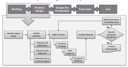
Figure 2 – Proposed sequence for VE systemic application – Process flowchart
