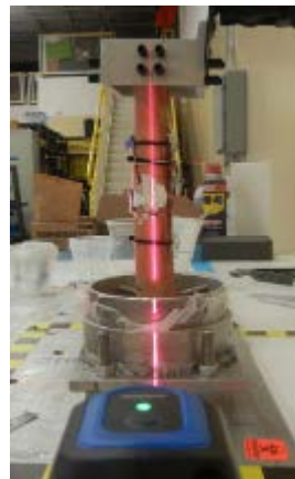
Fig. 7. Custom jig for aligning and potting the distal femur (left view)
