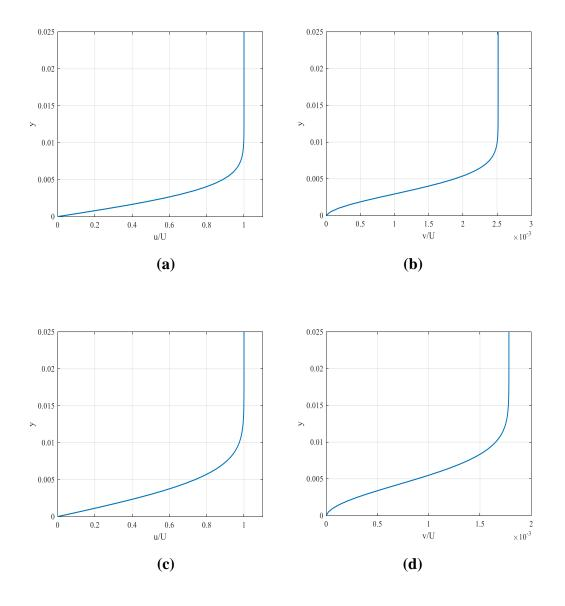
Figure 6.9 Numerical solution of the Oseen Boundary Layer equation at  $Re = 10^5$ .
