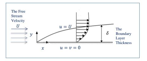
Figure 3.1 Velocity Boundary layer development on Flat Plate
