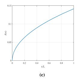
Figure 6.25 Boundary Layer Thickness of the Oseen-Blasius equation.
