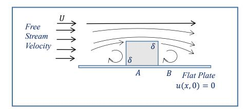
It could use the Finite Difference Method and the same Boundary conditions in Chapter 6 except on the flat plate it could be divided into 5 parts:
