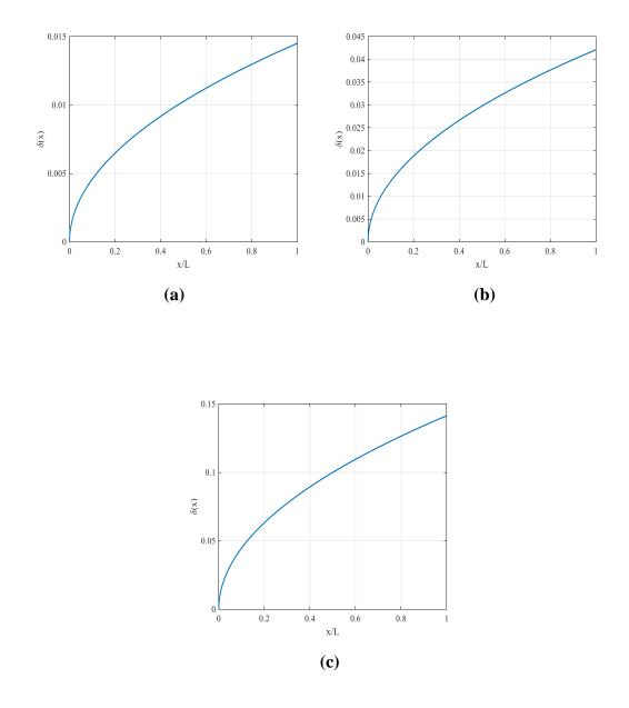
Figure 6.13 Boundary Layer Thickness  $\delta$  of the Oseen Boundary Layer equation.
