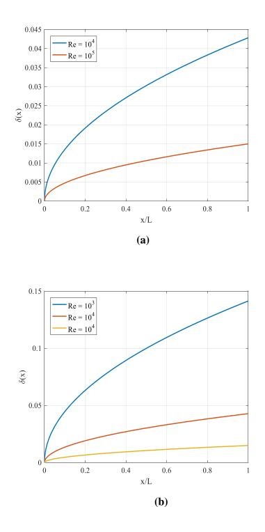
Figure 6.20 Boundary Layer thickness of Blasius equation in different Re.
