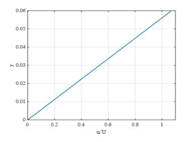
Figure 7.5 The solution of velocity *u* of Stokes boundary layer equation where x = 1 and  $Re = 10^3$ .
