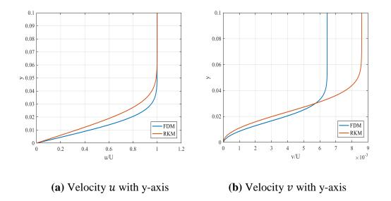
**Figure 8.11** Velocity of Blasius Equation at x=1 at  $Re = 10^4$  by RKM and FDM.
