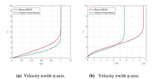
Figure 8.13 Comparison between analytic solution of Oseen-Blasius equation and Blasius solution by Runge-Kutta method at x=1.
