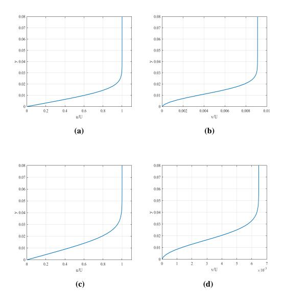
Figure 6.4 Numerical solution of the Boundary Layer equation at  $Re = 10^4$ .
