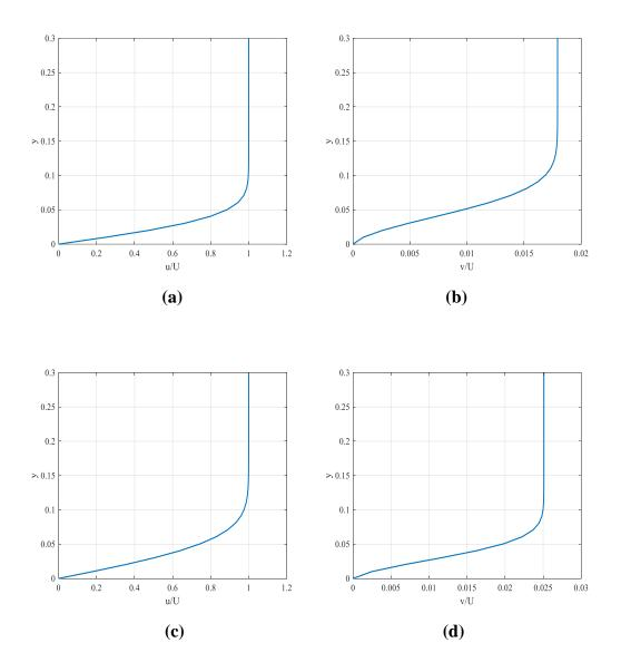
Figure 6.11 Numerical solution of the Oseen Boundary Layer equation at  $Re = 10^3$ .
