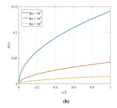
**Figure 6.8** Thickness  $\delta$  of Boundary Layer equation in different Re.
