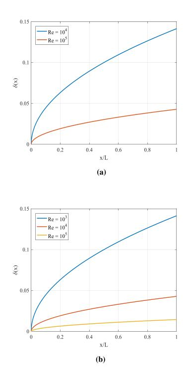
Figure 6.26 Boundary Layer thickness of the Oseen-Blasius equation in different Re.
