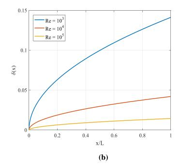
**Figure 6.14** Thickness  $\delta$  of The Oseen Boundary Layer equation in different Re.
