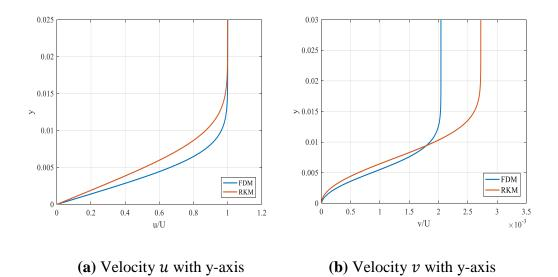
**Figure 8.10** Velocity of Blasius equation at x=1 at Re=10<sup>5</sup> by RKM and FDM.
