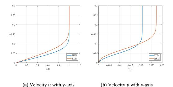
**Figure 8.12** Velocity of Blasius Equation at x=1 at Re=10<sup>3</sup> by RKM and FDM.
