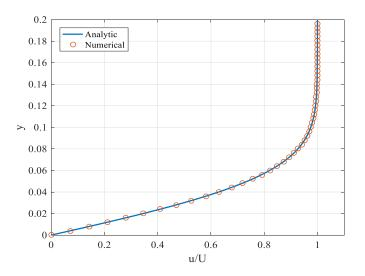
Figure 8.7 The x-momentum velocity u/U with y-axis of analytic and numerical solution of the Oseen-Blasius equation at x = 1.
