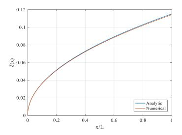
**Figure 8.9** The Boundary Layer Thickness  $\delta$  of analytic and numerical solution of the Oseen-Blasius equation.
