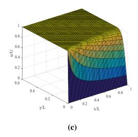
Figure 6.12 Velocity *u* Surface with *yx*-plane of the Oseen Boundary Layer equation.
