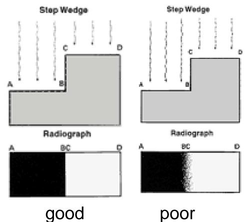
High definition: the detail portrayed in the radiograph is equivalent to physical change present in the part. Hence, the imaging system produced a faithful visual reproduction.
