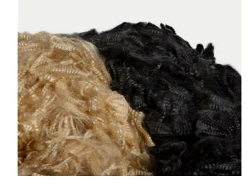
Available in either dark yellow or black, Technora® staple fibers reinforce textile applications for gloves as well as protective apparel against heat and cuts. These staple fibers are available with a specific fiber length of 51 mm, and a linear density of 1.7 dtex. In addition to staple fibers, Technora® can also be supplied as stretch broken yarns or as spun yarns, and with a linear density starting as low as 110 dtex.
