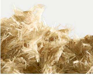
Technora® filament yarn can be converted into short-cut fibers or dipped chopped fibers with a range of lengths, typically between 1 mm and 30 mm, for use in, for instance, resin, cement and rubber reinforcement.
