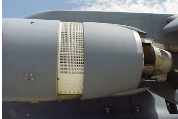
A deployed cascade reverser
