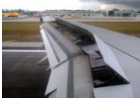
Ground spoilers deployed on an Airbus A321 (from http://en.wikipedia.org/wiki/Spoiler_(aeronautics) )
