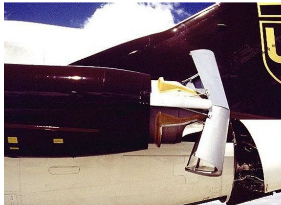
A deployed clamshell thrust reverser
