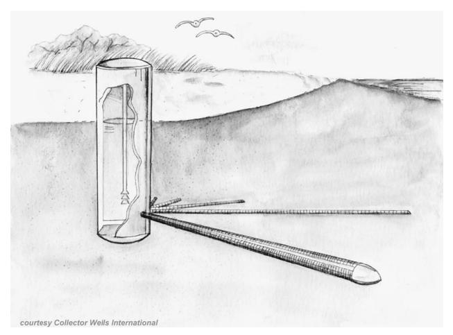
Figure 7 Radial well infiltration
