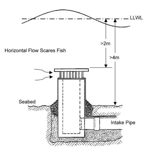
Figure 3 Velocity cap intake terminal
