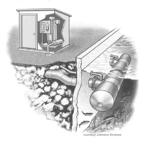
Figure 4 Passive screen seawater intake
