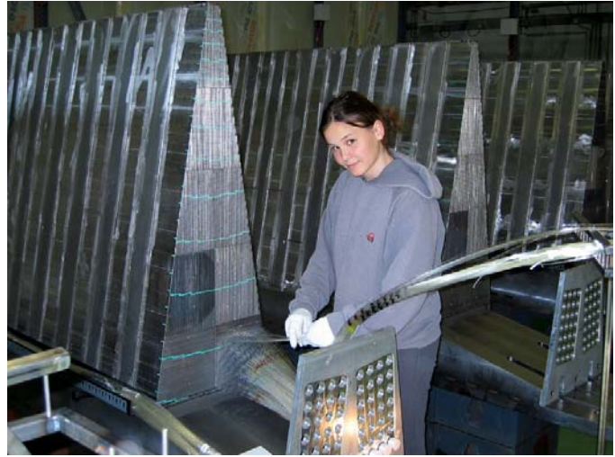
Fluorescence of wavelength-shifting fibres in plastic scintillator (left) and loading quartz fibres into an HF wedge (right)
