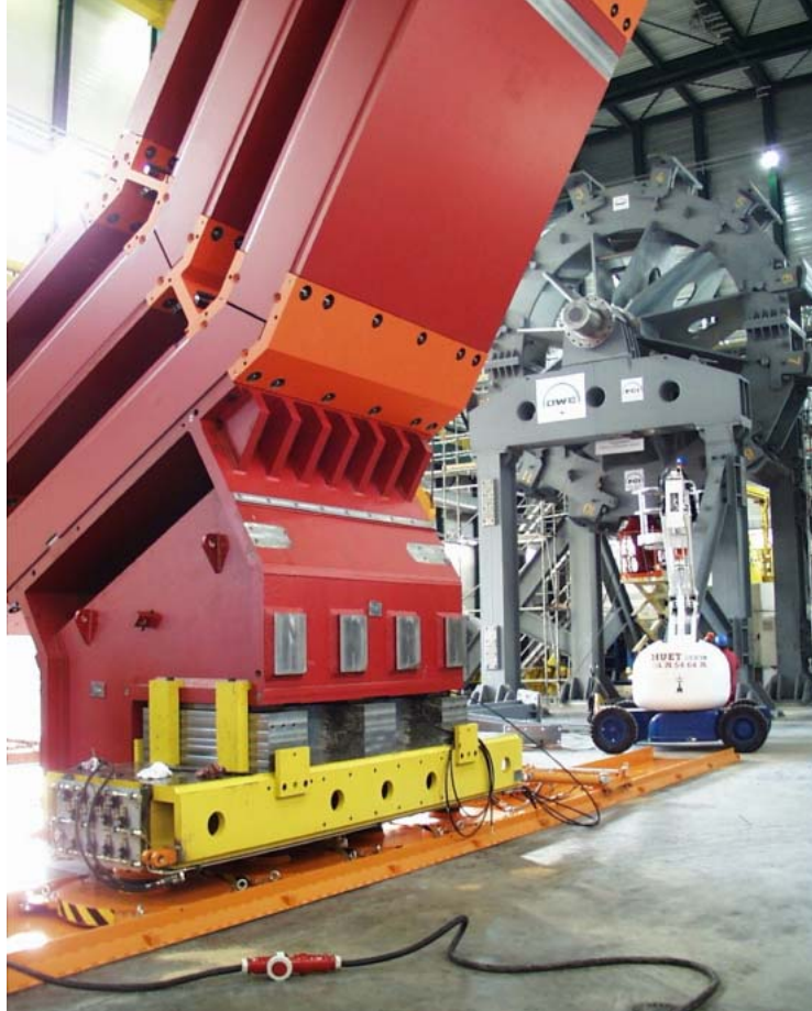
The air-pad system under the feet of one of the barrel yoke rings, used to move the large pieces of CMS around the surface hall
