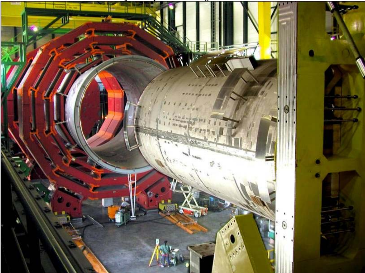
Trial insertion of the inner vacuum vessel using the rotating platform. The inner vacuum vessel is currently in the vertical direction (November 2003)
