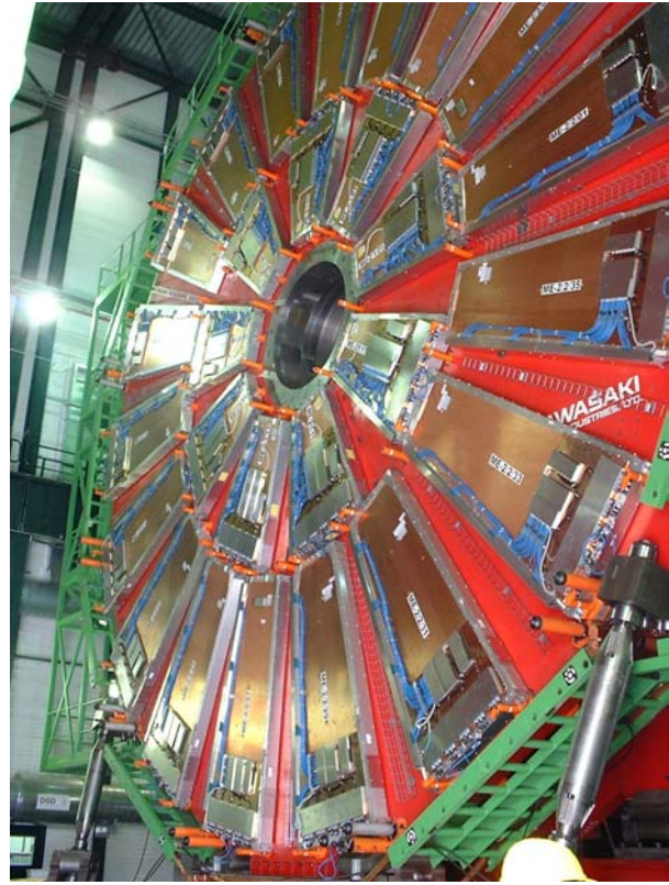
One endcap disk loaded with muon chambers
