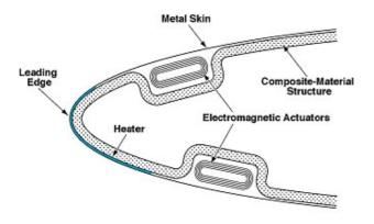
Fig.4 Electro-Expulsive Deicer located in the wing nose – a possible arrangement
