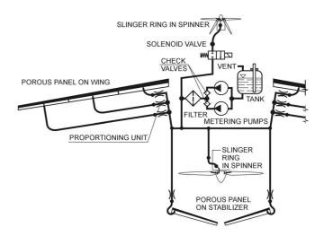
Fig.12 Ice Protection Fluid System proposed for MALE UAV, developed at Warsaw University of Technology
