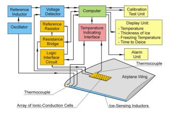
Fig.14 Ice thickness monitoring system developed at NASA Ames, US Patent No. 5,523,959
