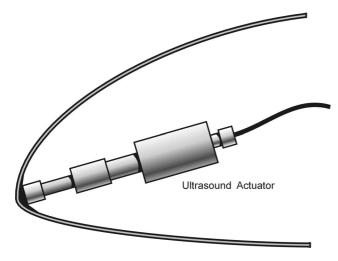
Fig.11 Ultrasound actuator placed inside the nose of leading edge
