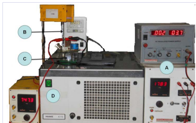
Figure 1a: Experimental set up for Electrodeposition (A) Regulated DC power supply (B) Stirrer (C) Electrolysis cell consisting of two nickel anodes and a copper cathode and (D) a thermostat to maintain the constant bath temperature.
