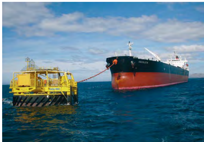
Gambar 2.1 Single Point Mooring ( www.marineinsight.com )
